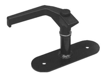
This easy to operate window handle is designed to fit comfortably in the hand for top and side hinged windows for on and off-highway vehicles. Featuring 90 degree rotation with steel mounting plate and glass filled nylon handle.
